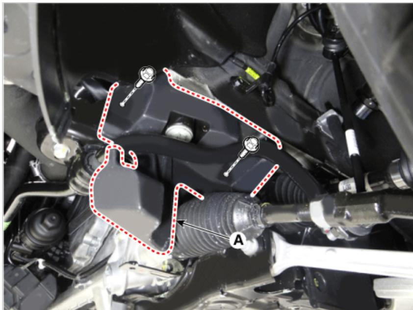
3. Remove the engine room rear side cover (A).
